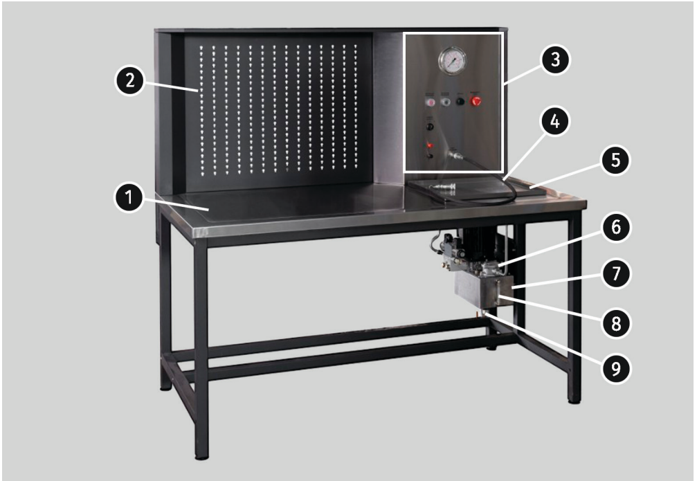
Figure 1. Main elements of the bench
